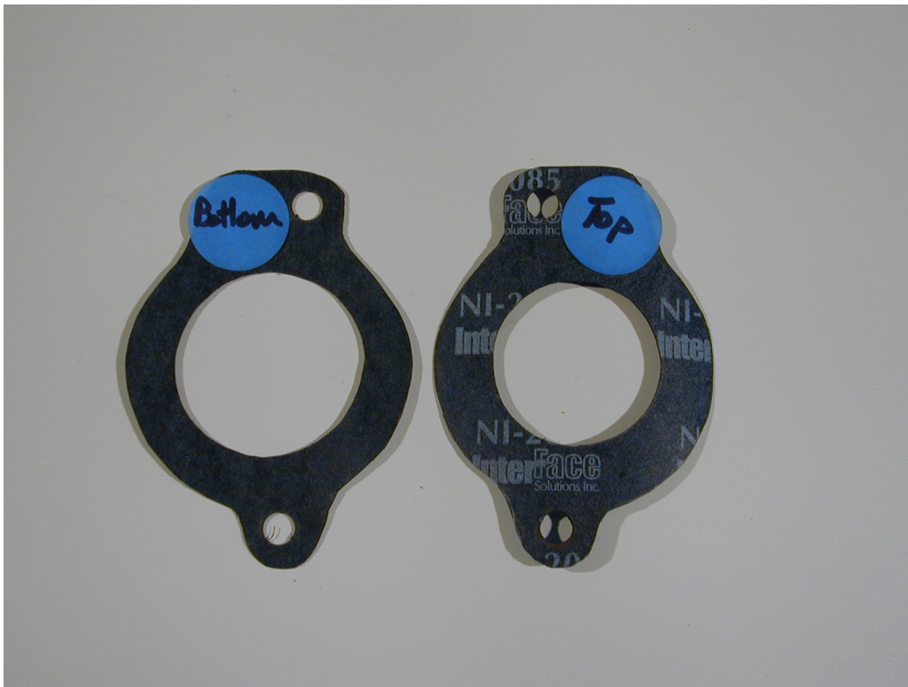
Figure 10: Top and Bottom Gasket Configuration
