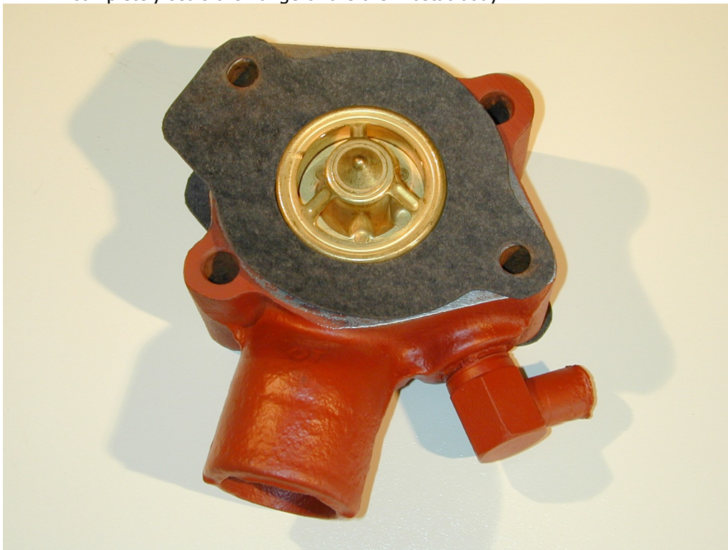
Figure 11: Top Gasket to Thermostat Installation
