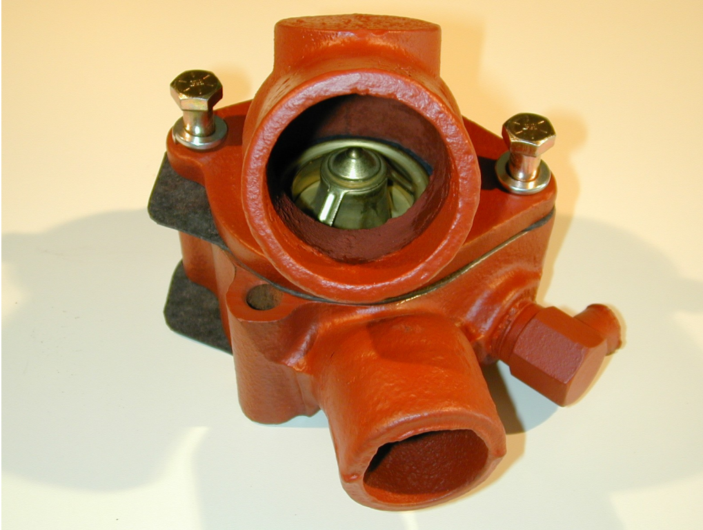
Figure 3: Early SV Water Neck, Thermostat Housing, Thermostat, and Gaskets/Fasteners
