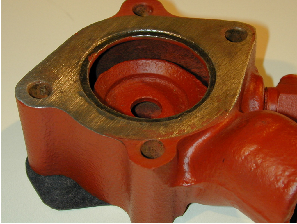
Figure 4: Thermostat Housing Counter-bore
