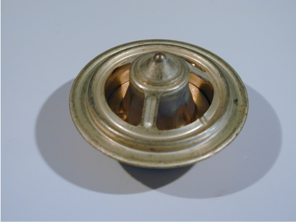
Figure 8: Air Bleed Formed in Thermostat Body at 5 o'clock Position, Top View
