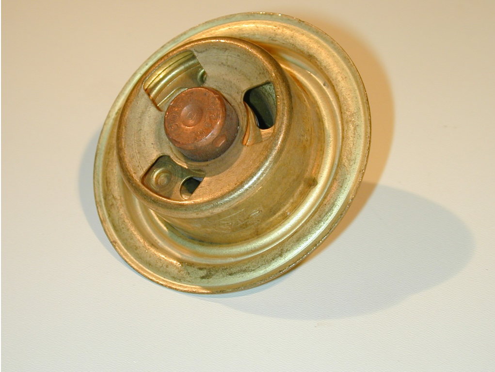
Figure 9: Air Bleed Formed in Thermostat Body at 4 O'clock Position, Bottom View
